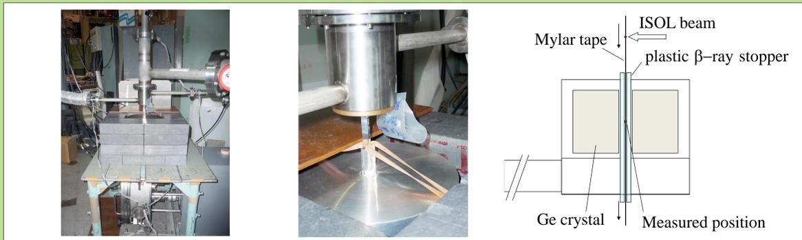
Photographs (left and center) and a schematic drawing (right) of experimental setup at KUR-ISOL.
